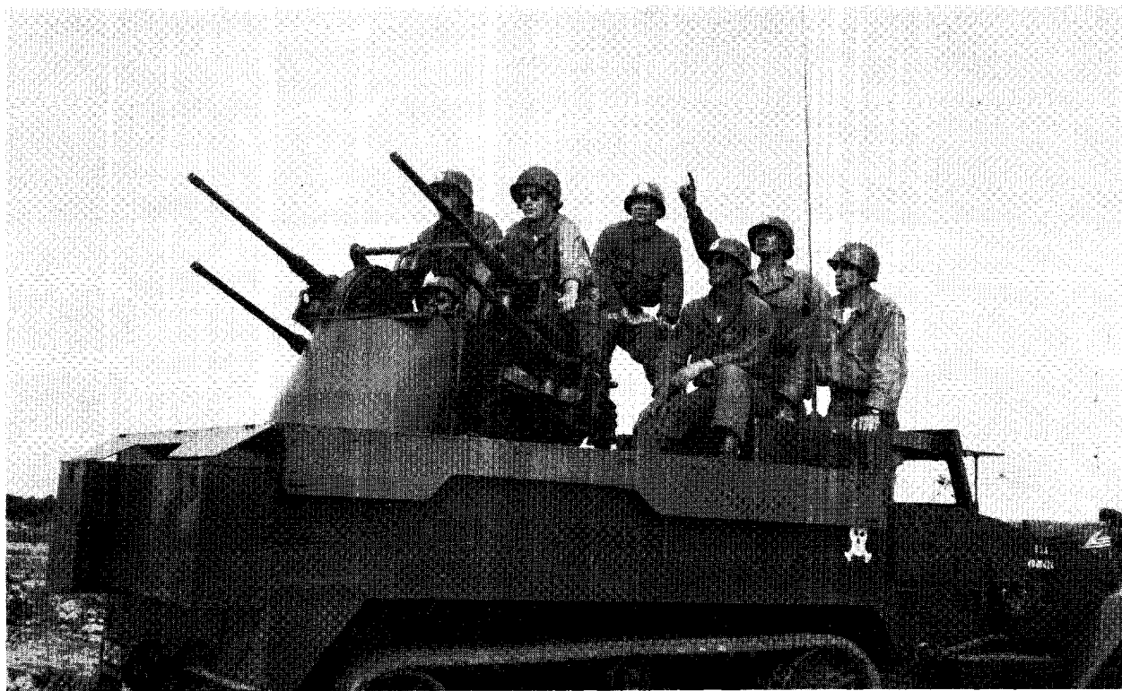
M-16 half-track with multiple 50 caliber machine guns mounted, issued to anti-aircraft artillery automatic weapons battalions (self propelled), organic with division artillery
