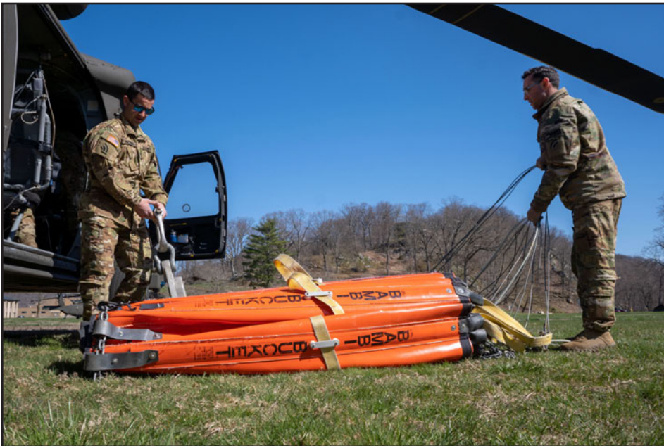
Army aircrews from the 3rd Battalion, 142nd Aviation conduct water bucket training at Camp Smith Training Site April 6, 2021. Water Bucket training tests equipment functionality to prepare aircrews to be ready to fulfill state fire suppression needs, while providing necessary qualification for helicopter pilots.
