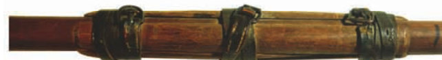
Wooden splints and leather straps are used in a field repair to reinforce a damaged staff.
