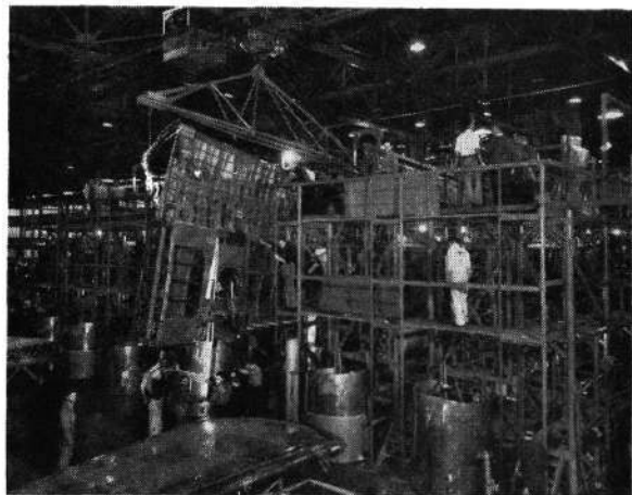
BIRTH OF A FLYING FORTRESS WING: A B-17B wing panel, with engine nacelles attached, emerges from its construction jig. The crane which carries it can be seen above. The picture shows part of the series of massive steel jigs in which the bomber wings are assembled, at Boeing Plant No. 2. Elaborate scaffolding enables the assembly crews to work at several different levels as well as on the top and bottom of the wing surfaces simultaneously. The completed Flying Fortress wings will support more than 100 tons.
