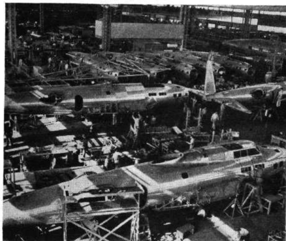
ALONG THE FLYING FORTRESS PRODUCTION LINE: These Boeing B-17B bomber bodies, assembled in a series of steel jigs in another section of the plant, take their place at the start of the final assembly line. After each has received its wings (on which the landing gear has already been installed) it is rolled forward to a new position in the line on its way to completion. The body in the middle of the picture is just being lowered by overhead cranes to its place on the assembly floor.
