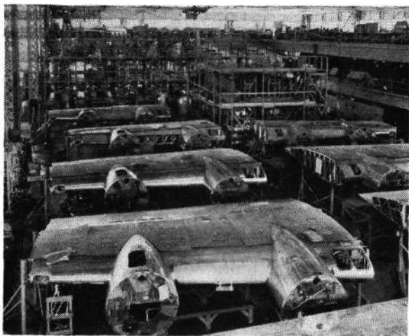
BIRTH OF A FLYING FORTRESS WING: A B-17B wing panel, with engine nacelles attached, emerges from its construction jig. The crane which carries it can be seen above. The picture shows part of the series of massive steel jigs in which the bomber wings are assembled, at Boeing Plant No. 2. Elaborate scaffolding enables the assembly crews to work at several different levels as well as on the top and bottom of the wing surfaces simultaneously. The completed Flying Fortress wings will support more than 100 tons.
