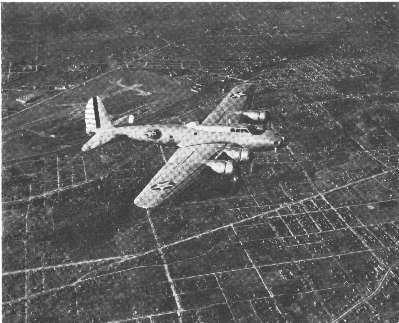
Flying Fortress for Substratosphere: First photograph of the new Boeing YB-17A Flying Fortress, which has special engine superchargers for operation in the substratosphere. Built by the Boeing Aircraft Company for the United States Army Air Corps, this advanced Flying Fortress is now undergoing tests. It is a 22-ton four-engine bomber similar in general design and identical in size to the Boeing B-17 Flying Fortresses now in Army service.
