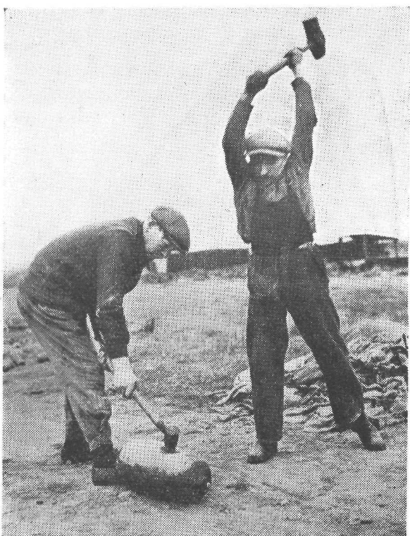
● Perforating a smoke bomb before firing its contents.
