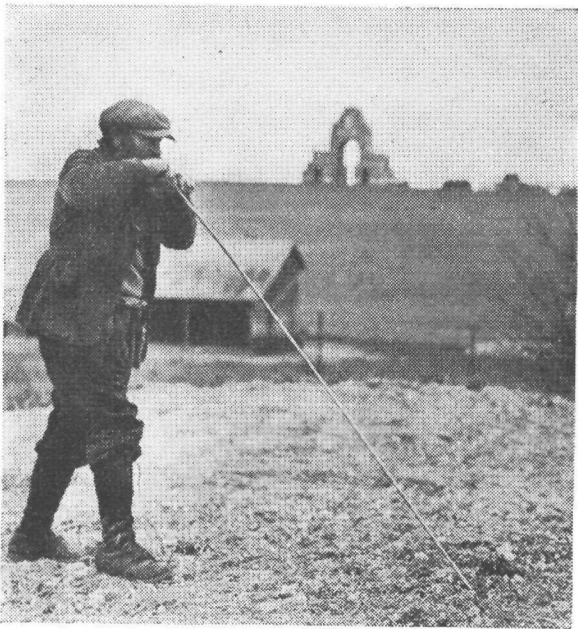
● Probing the ground with a long metal rod tipped with a highly polished point. Contact with a hard body leaves a trace on this point which indicates whether the object is brass, copper, steel or stone.
