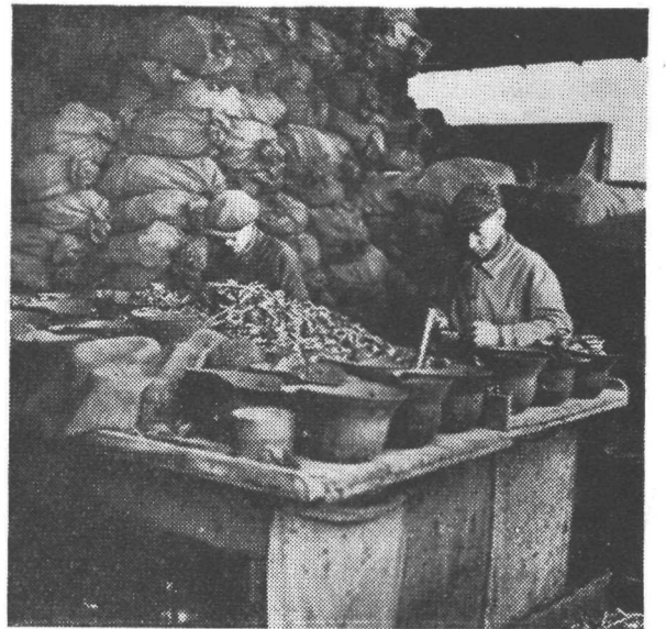
● Sorting small parts as to classification — zinc, brass, copper, aluminum, etc.
