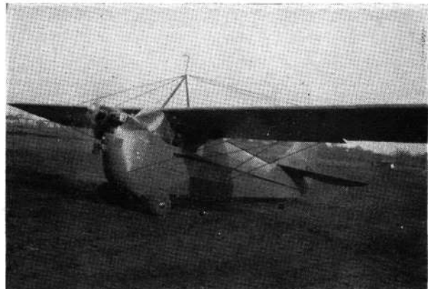
Two excellent views of the Orion Flying Club's new Aeronca two-place, side-by-side, high-wing monoplane. The cabin is heated for winter flying and can be opened up when the weather permits. Note the safe landing gear and the deep, roomy body.
