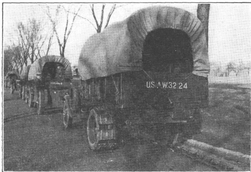
**A** REAR view of the truck column. Battery personnel, as well as ammunition, are carried in the trucks. The shoe-plates, as illustrated, are readily attached to the rear wheels for travel over difficult terrain.
