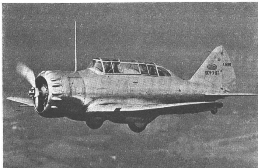
The introduction of aircraft into warfare gives a commander-in-chief a new means of reconnaissance and enables him to take a stronger offensive against vital lines of supply and communication. The above machine is a Seversky advanced trainer for combat and tactical work, capable of speeds well over 200 m.p.h.
