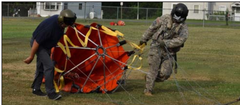
Staff Sgt. Jimmy Rose (right), assigned to the 3rd Battalion, 142nd Aviation, and civilian Steven Rosen, load a Bambi bucket onto a UH-60 Blackhawk Helicopter in Altona, N.Y., July, 13, 2018 during firefighting operations.
